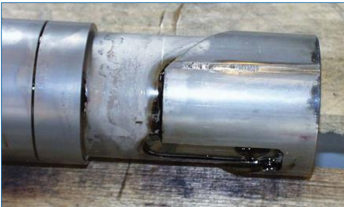
Fig. 2: Damaged plunger of injection pump
