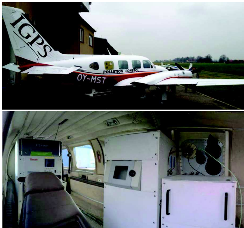
Figure 3. The ship surveillance system installed in a Danish Navajo Piper aircraft (OY-MST) (upper). To the left the gas rack is shown, in the middle the particle rack (Not applicable here) and on the right side the optical rack. In the upper right part of the picture a probe plate is shown containing telescopes and sondes.
