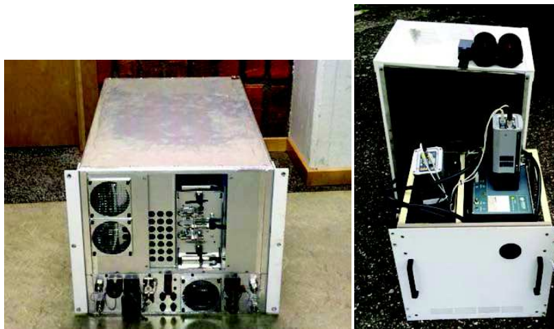
Figure 4. The ship surveillance system installed in a Danish Navajo Piper aircraft (OY-MST). To the left the custom made sniffer module is shown which includes all necessary hardware to carry out FSC compliance measurements from the air, i.e. logging computer, AIS receiver, GPS receiver, power converter, calibration gases, fluorescence SO 2 -sensor, NDIR CO 2 -sensor and pressure regulators (47 kg, 15 A). On the right side the optical rack is shown, (5 A, 30 kg).
