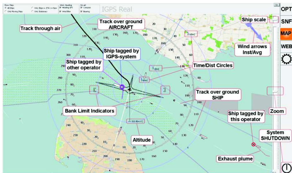
Figure 2. A screenshot from the program IGPS real when flying. The software utilizes information from AIS and GPS receivers and wind speed and direction to plot the location of the aircraft, ships and their exhaust gas plumes.
